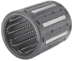
Linear ball bearings are available in compact LBB range (ISO series 1) and standard LBC range (ISO series 3). The bearings consist of a polymer cage with steel raceway segments to guide and recirculate the ball sets within the complete cage. The range is available with or without seals, in standard and open types as well as in corrosion resistant versions.
