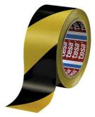
tesaflex® 60760 is a tough plasticized PVC tape coated with an aggressive modified rubber-resin adhesive, which allows adhesion on many different surfaces. tesaflex® 60760 is even tearable by hand.
