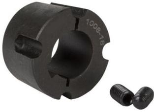
Fenner Taper Lock® bushes are machined in cast iron and steel and are available in a full range of both metric and Imperial bores and keyways. They have the equivalent to a shrink-on fit on uniform load applications and offer complete ease of installation and removal. The special 4-hole feature on Fenner Taper Lock® bushes is a feature for balanced assemblies.
