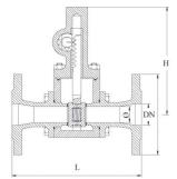
Wedge material: Aluminum bronze Suitable for continuous discharge: No Maximum pressure at 20 °C: 40 bar Maximum pressure at 400 °C: 21 bar
