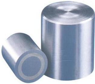
Design: Made of AlNiCo 500. In smooth design with fitting tolerance of h 6. Steel housing, well shielded. Max. operating temperature is max. 450 °C. Overall length  $l$  can be shortened by  $h$  with no loss of holding force.
