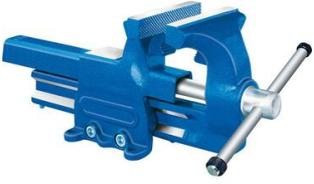
Design: Solid design, fully steel-forged with hardened surface. Jaws and anvil surface-hardened (54?58 HRC), anvil surface suitable for straightening and compression work; front-opening. Precise clamping thanks to adjustable bearing, with double-trapezoid thread for rapid clamping of workpieces, cover protects against penetration of metal dust and other foreign particles. With welded pipe-clamping jaws.
