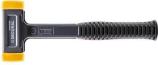
Design: Hammer body made of sturdy sheet steel, the interchangeable, medium hard impact heads are made of cadmium-free, yellow polyurethane. Kickback free through ball filling. Handle coated with ergonomic rubber sleeve.
