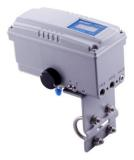
Transmission: Linear Execution: Positioner Function actuator: Single acting Input signal: 4 - 20 mA Level of protection (IP value): IP66 Electrical connection: 1/2" NPT gland nut Display: Yes Stroke: 16 to 30 mm With console: Yes Standard actuator connection: DIN IEC 60534-6-1 With assembly set: Yes Material housing: Aluminium Material konsole: Steel
