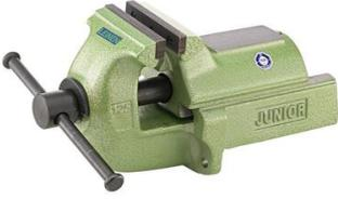
Design: Heavy, solid design made of high-strength grey cast iron, the best clamping precision thanks to the long and precise dovetail guide. Concealed, dirt-proof and smooth-running acme thread spindle, interchangeable and reversible hardened steel jaws, integrated pipe clamping jaws, opens to rear and with large anvil surface for simple straightening work.
