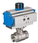
The pneumatically operated 2-way ball valve is configured according to the following basic principles: Pneumatic pilot pressure at 6 bar, medium is water, medium temperature is max. 100°C, ball valve is actuated at least a few times daily, actuator structure according to Eriks standard.
