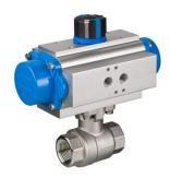
The pneumatically operated 2-way ball valve is configured according to the following basic principles: Pneumatic pilot pressure at 6 bar, medium is water, medium temperature is max. 100°C, ball valve is actuated at least a few times daily, actuator structure according to Eriks standard.
