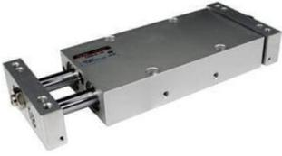
Slide unit series CXW can absorb energy in a wide range, in high-speed, low-load applications to low-speed, high-load applications, without requiring adjustments. The slide unit can be mounted on the housing or on the plate, depending on the application. Slide bearing or ball bushing bearing is available. Auto switches can be installed.
