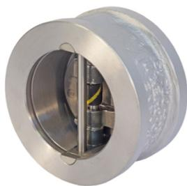
Crane Stockham Duo-Chek stainless steel wafer type, dual plate check valve, according API 594. Metal seated, suitable for mounting between ASME B16.5 RF Class 600 flanges.
